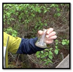
We are looking at the **pH** of the water. What does pH mean? It's a measure of how much acid is in the water. The range goes from 0 to 14, with 7 being neutral. We would expect the pH of a natural water area like this to be between 6 and 8. To test, an "indicator" interacts with the water sample causing the water to change color depending on the pH. We then compared the color in the bottle to the pH color chart.
